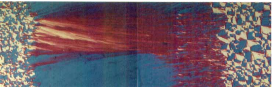
Figure 5. Optical texture (crossed polarizers; \lambda -plate) of the contact zone between 10a and 7c at 100°C.
